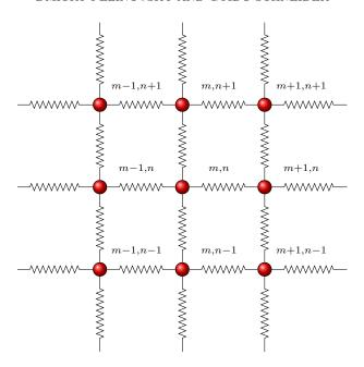
Fig. 1. A mass-spring system arranged in a 2D square lattice. The masses are fixed at the (m,n) sites with the vertical displacements given by  $q_{m,n}(t)$ .
