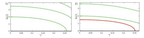
Fig. 3 Purely imaginary eigenvalues  $\lambda$  of the  $\mathcal{PT}$ -symmetric problem (30) for the first two stationary states with  $\mu=12$ . Eigenvalues of negative (positive) Krein signature are shown in red (green), complex eigenvalues are shown in black
