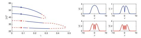
**Fig. 2** Left: Power curves for branches of nonlinear states for  $\mu=12$  and  $\gamma>0$ . Solid blue (dashed red) curves indicate stable (unstable) states. Right: Sample profiles for nonlinear states that correspond to the points shown on the power curves, from the top to the bottom branches
